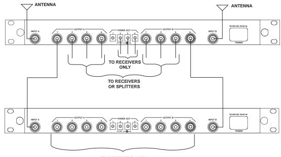
TO RECEIVERS ONLY (DO NOT FEED SPLITTERS FROM SECONDARY UNITS)
